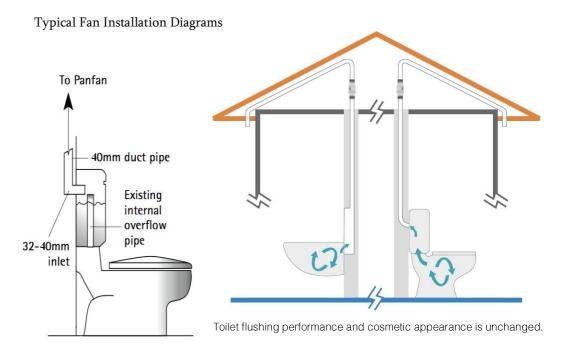
IMPORTANT: ALL PIPE WORK MUST FALL TO AN OUTLET TO DRAIN ANY CONDENSATION.
